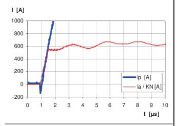
Fast increasing currents (higher than the specified  $I_{p,max}$ ), e.g. in case of a short circuit, can be transmitted because the currents are transformed directly and be limited by diodes only.
